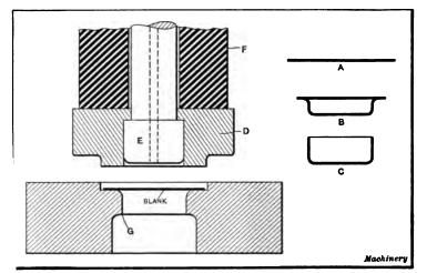
Fig. 7. Plain Drawing Die equipped with Blank-holder
